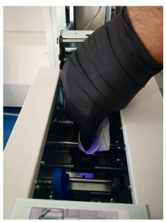
a) First press the soaked cloth against the upper roller and then press one of the two upper right buttons at the front panel:
