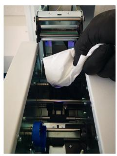
c) If yes, repeat the procedure with a clean part of the cloth. Check the cloth again. If it is only light grey the roller is cleaned. Repeat at your own discretion.
