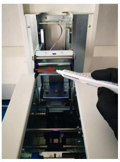
4. If the cleaning pen does not resolve the issue, the pink cleaning cloth (Printhead Polishing Paper: 895703DTM) should be used. Rub the cleaning cloth over the printhead burn line a few times to help remove any built-up debris.
